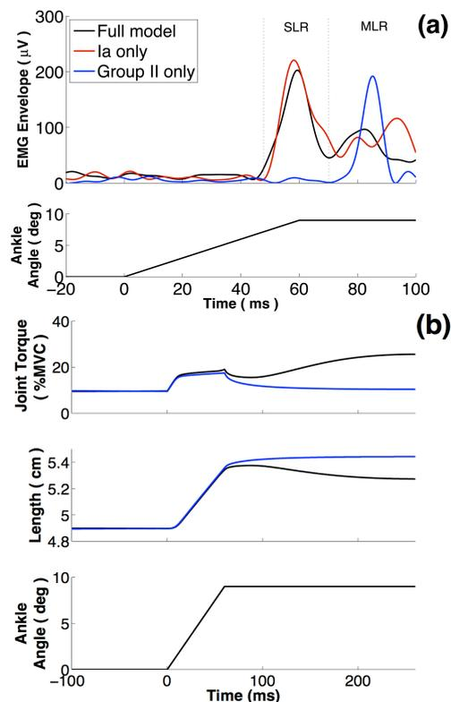
**Figure 2:** Simulation input and output signals. **(a)** EMG envelope of the SO muscle and ankle angle (input). Black, red and blue curves represent three different simulated conditions (see Methods). **(b)** Ankle joint torque, SO muscle length, and ankle angle (input). Black curves have a reflex contribution, whereas the blue curves represent the passive (no reflex) behavior. The horizontal scale is different in (b).
